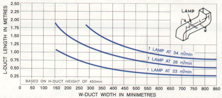
Figure 6 Number of AeroNomics MS14 U.V. lamps required for 80% kill of microorganisms in air ducts.
